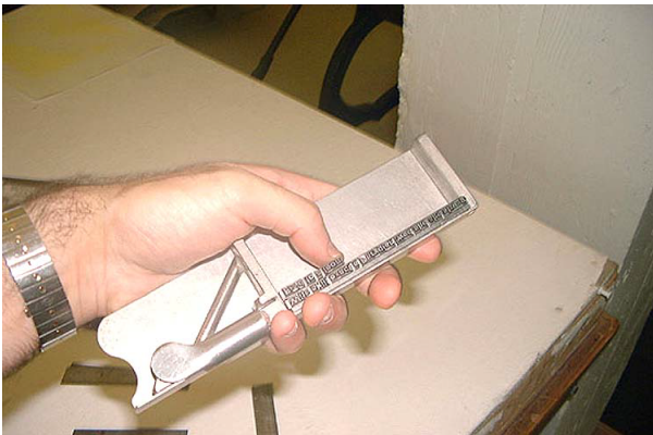
Typical character: Notice these were solid metal and there was no way to set them closer to another character, in width or height.
